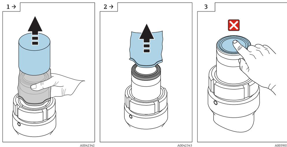
Check that the seal is seated correctly. If necessary, position the seal properly.
