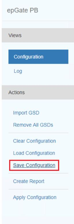
The configuration is automatically saved on the Laptop in a \*.json file, called "PROFIBUS-Cfg.son". **It is recommended to save the PROFIBUS configuration because after a reboot of the epGate PB gateway the Web server PROFIBUS configuration is not displayed anymore.**
