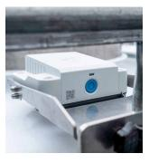
Micropilot FWR30 mounted on an IBC
