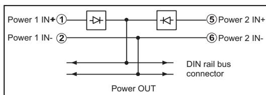
Block diagram power terminal block
