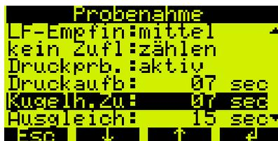
Under Set-up – Unit settings – Sampling – Press. samp. the option can be selected.
