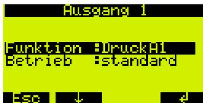
Under Set-up – Unit settings – Outputs – Output 1-3 can be selected as pressure output A1.
