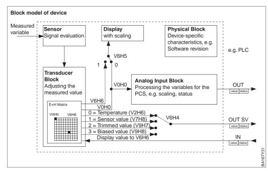
Figure 3.3 Block model of the Deltabar S with PROFIBUS-PA profile 3.0
