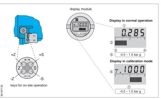
Figure 4.1 User interface of the Deltabar S, with optional display
