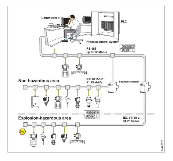
Figure 3.1 PROFIBUS-DP/-PA principle of operation
