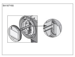
• Insert the plug of the display in the centre jack. Note the coding of the plug and jack.
