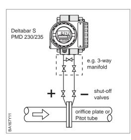
Measurement with orifice plate or Pitot tube
