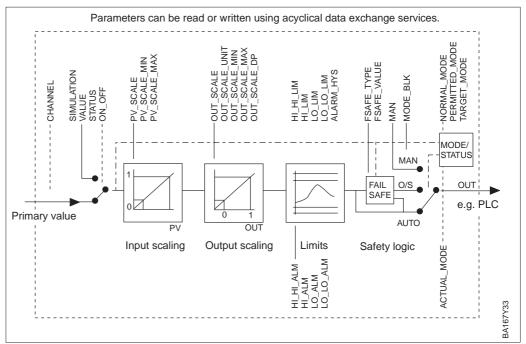
Figure 3.4 Schematic diagram of the Deltabar S analog input block The device parameters are listed in the following tables. The parameters are accessed via the slot and index number. The analog output, transducer and physical blocks contain standard parameters, block parameters and manufacturer-specific parameters.
