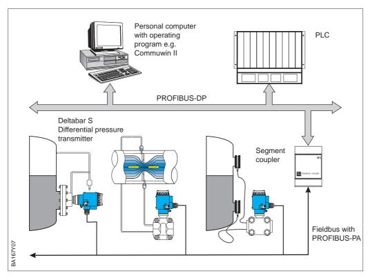
Figure 1.3 Measuring system Deltabar S with PROFIBUS-PA protocol
