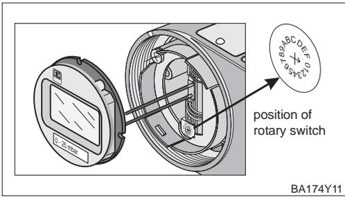
After calibration, a characteristic curve for the output signal must be selected according to the application. The setting is done with the rotary switch which can also be used for damping.
