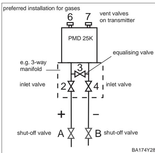
The three-way manifold comprises two inlet valves and an equalising valve.
