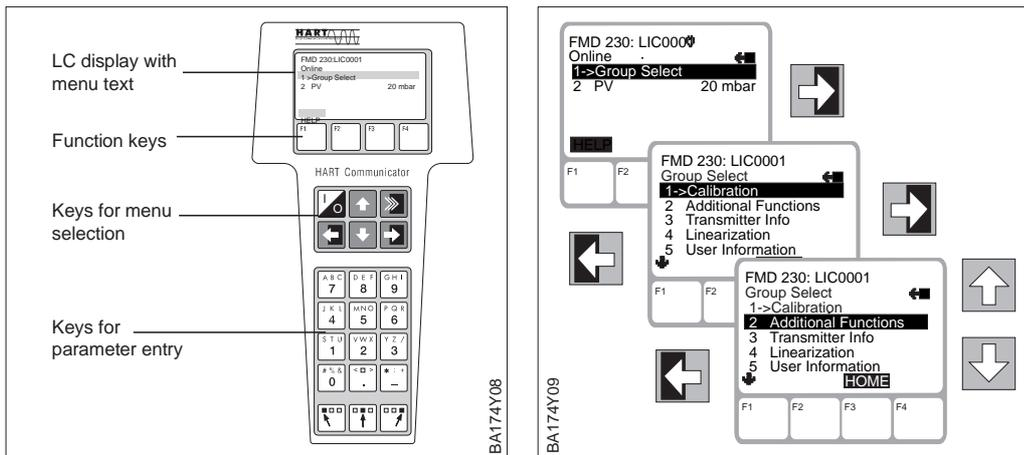
If the HART protocol is used, the device is operated via a menu which is derived from this matrix, see manual for handheld terminal.
