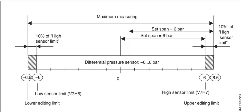
**Example of editing limits for a differential pressure sensor -6...+6 bar**
