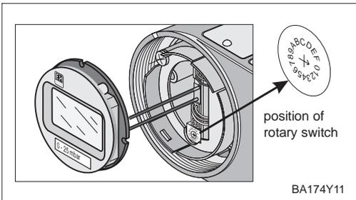
Set the blue damping switch to "0". The transmitter can only be operated by the handheld terminals or the Commuwin II operating program when in this position.
