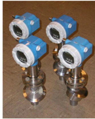
FMP 40's with modified mounting, ready for probe connection and tank installation
