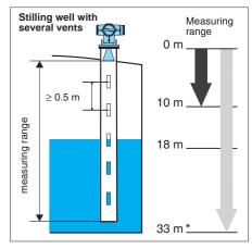
Max. vent diameter DN 80/3": 20 mm ≥ DN 100/4": 25 mm
