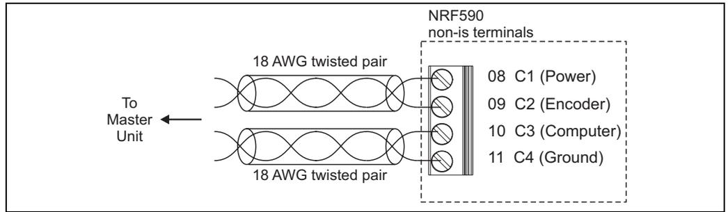
Fig. 1: Wiring diagram for L&J Tankway Protocol
