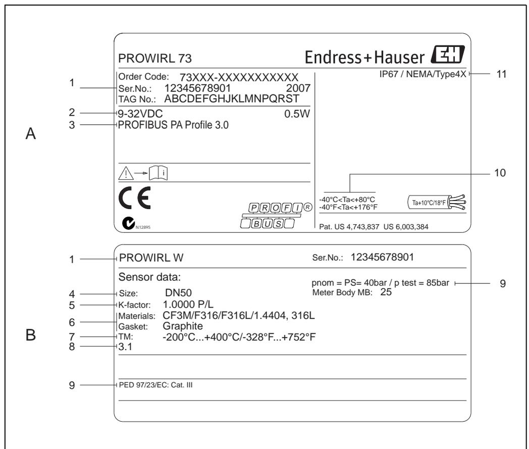
Fig. 1: Nameplate specifications for transmitter and sensor (example)
