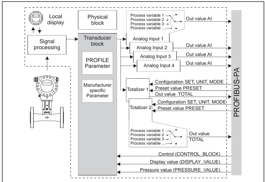
Fig. 31: Block model Proline Prowirl 73 PROFIBUS PA Profile 3.0
