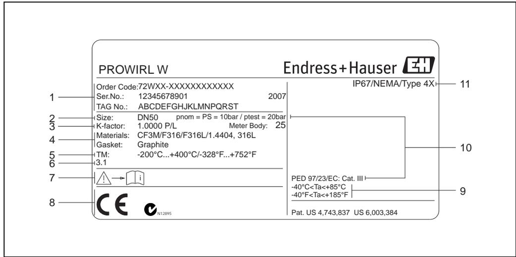
Fig. 2: Nameplate specifications for transmitter, remote version (example)
