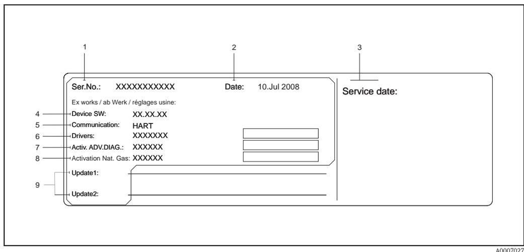
Fig. 3: Service nameplate specifications for transmitter (example)
