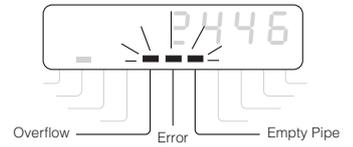
Errors which occur during normal operation are indicated on the display by appropriate *segment bars* ("Error, Empty Pipe, Overflow").
