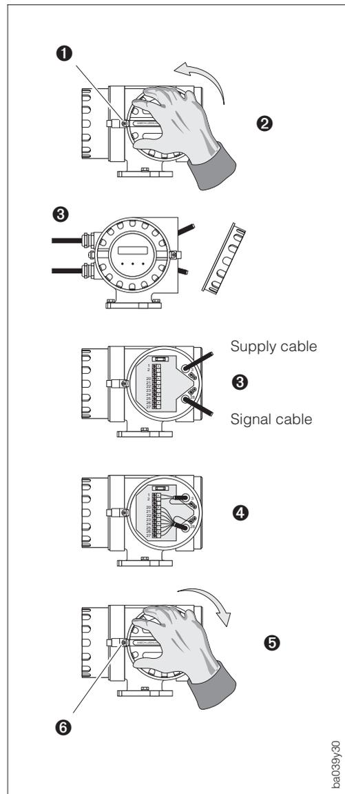
1. Loosen the Allen screw of the safety grip using a 3 mm Allen key.
