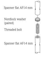
The following tools are required for mounting the rod parts:
