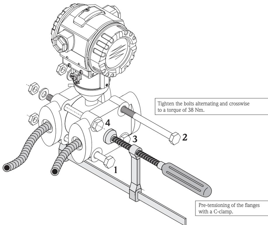
**Hints for disassembly / assembly of a sensor assembly**
