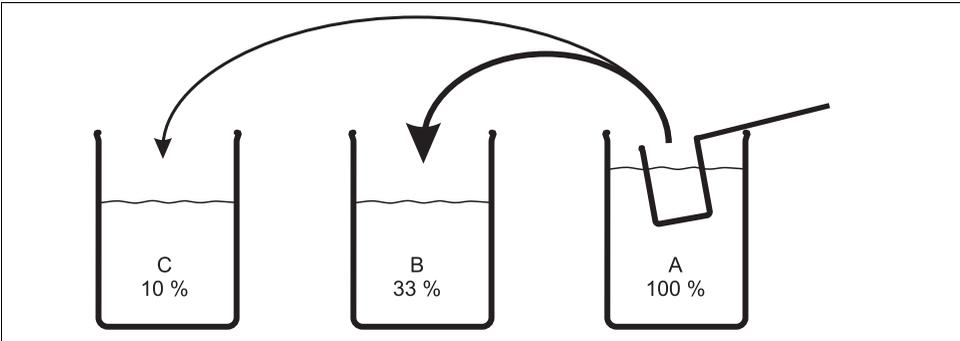
Fig. 8: Creating samples for a three-point calibration
