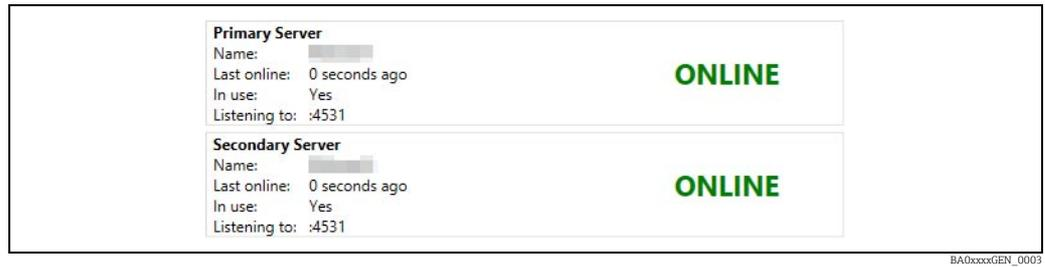
The primary and secondary servers are both online in a redundant configuration.
