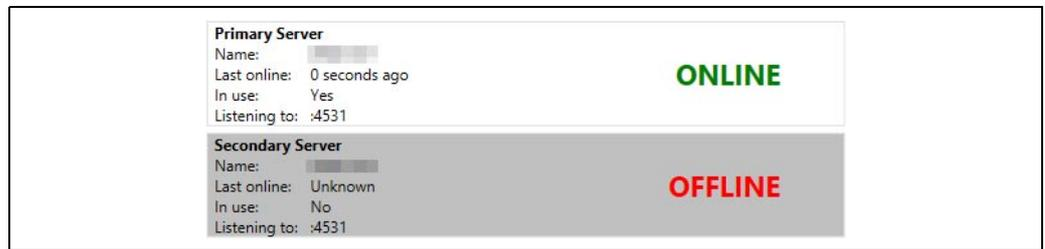
A user has switched the configuration to a single-server configuration after the secondary server went offline.
