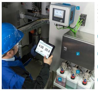
Liquiline Control CDC90 cleans, validates, calibrates and adjusts pH electrodes fully automatically.
