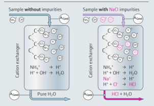
The **total conductivity** is measured upstream from the cation exchanger. In the exchanger, all the cations are replaced by H<sup>+</sup> ions. If the water does not contain impurities (example on the top left), the result is pure water with a lower conductivity downstream from the cation exchanger.
