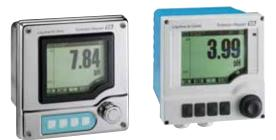
Liquiline CM14 The four-wire transmitter for pH/ORP, conductivity and oxygen is an instrument for basic measurement requirements. Handling is easy, though CM14 does not share hard- or software with other Liquiline devices. The compact design of Liquiline CM14 is suitable for installation in panels or cabinets and especially attractive for skid building in:
