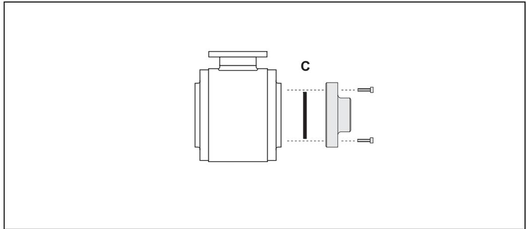
Promag H process connections (DN 40 to 150, 1½ to 6")
