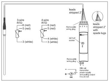
Wiring example - wiring with DIN rail transmitter TMT 121
