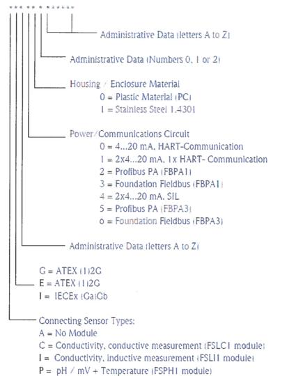
L = Digital Sensor Inductive Conductivity, MEMOSENS (FSDG1 module)
