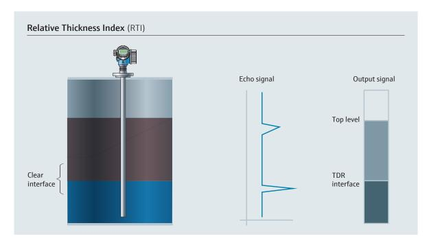
At a clean interface of water and condensate the Relative Interface Echo Amplitude is higher than 70mV.
