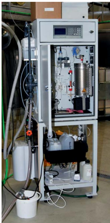
The CA72TOC checks the organic load in the wastewater during cheese production.
