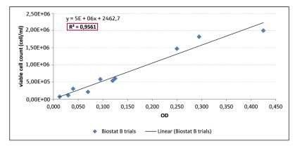
Example of the correlation for the 5 litre bioreactor in the lab (several batches).
