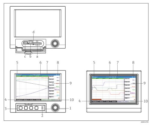
Device front (left: version with navigator and front interfaces; right: version with stainless steel front and touchscreen)
