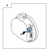
If the main board is replaced, store the DAT module in a safe place until it is installed in the new electronics module. It contains all of the data on the device and measuring point.
