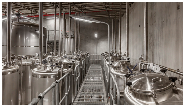
Spirits storage tanks with Endress+Hauser with Micropilot FMR52 for level monitoring
