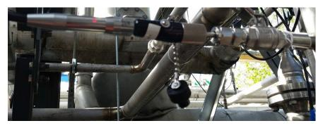
In-line chemical analysis of amine process stream by a Raman immersion probe at the  $\rm CO_2$  capture plant facility in Sheffield, UK
