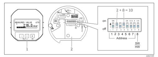
Fig. 8: Setting the device address via DIP switches
