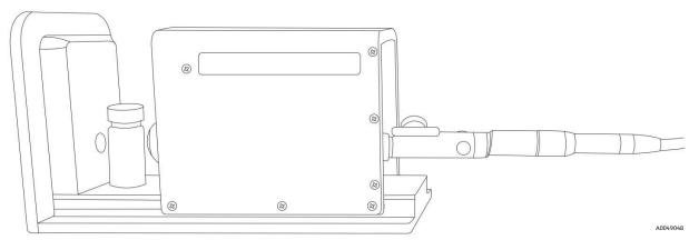
$Figure\ 3.\ Enclosed\ Sample\ Compartment\ with\ sample$
