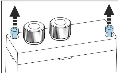
Loosen the Allen screws (AF4) of the cover and then remove the cover.
