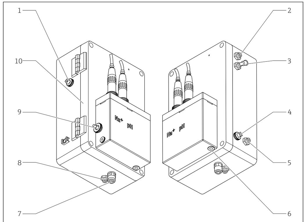
2 Liquid control unit including measuring unit and supply vessel
