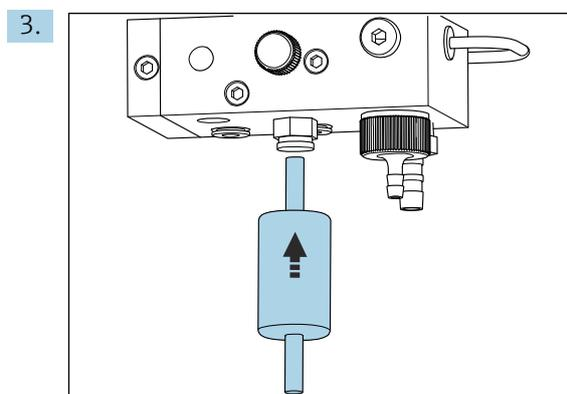
Insert a new filter cartridge, while paying attention to the flow direction (indicated on the adhesive label on the filter)!
