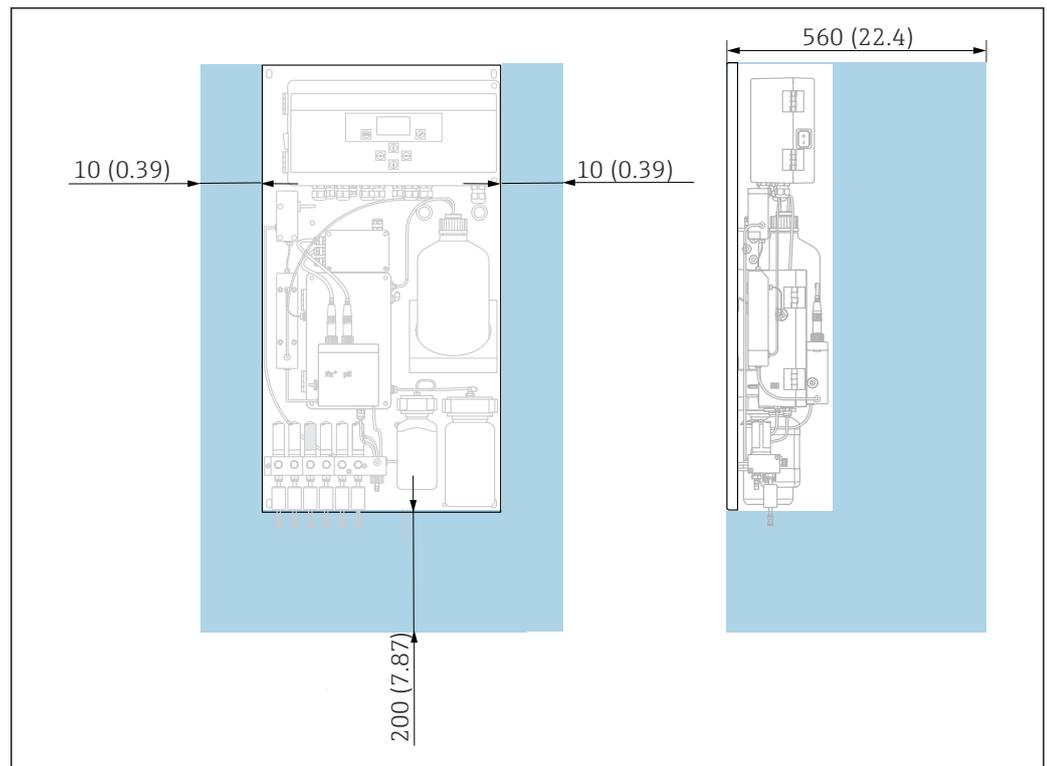
5 Analyzer CA76NA, spacing requirements in mm (in)
