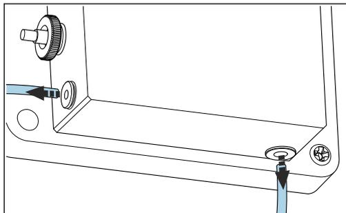
Untighten the hose connections of the measuring unit. To do so, gently squeeze the hoses in the direction of the connector, while pressing the locking ring, and remove the hose from the connector.
