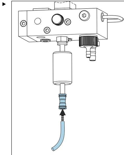
Connect sample hose using quick-release coupling.
