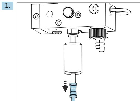
Remove the medium supply hose with a quick-release coupling at the filter.
