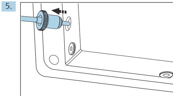
Remove the temperature sensor fitted on the left-hand side of the measuring unit, while making sure you do not lose the O-ring fitted in the measuring unit.
