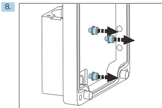
Hold the measuring unit steady and loosen the three securing screws on the inside of the cover of the liquid control unit with an Allen key (AF4).
