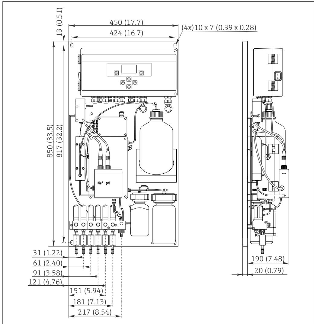
4 Analyzer CA76NA. Unit of measurement mm (in)
