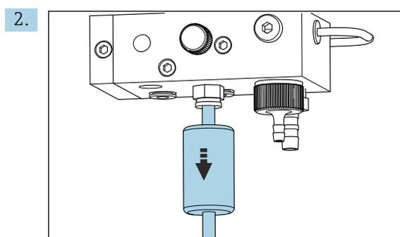
Remove the filter cartridge.
