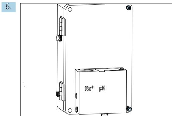
Loosen the 2 PH2 Phillips screws on the cover of the liquid control unit and open the cover.
