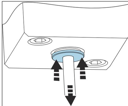
Hoses can only be removed when unpressurized:
