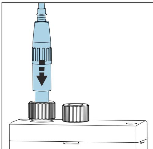
Carefully insert the electrode as far as it will go into the left-hand chamber (sodium) or right-hand chamber (pH).
