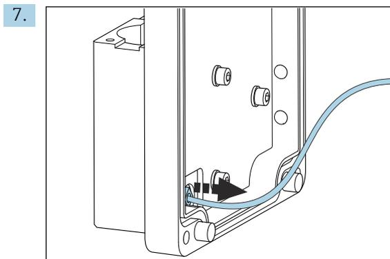
Unscrew the hose to the circuit pump.
