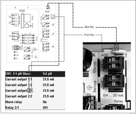
Slot and port assignment of hardware and presentation on the display
