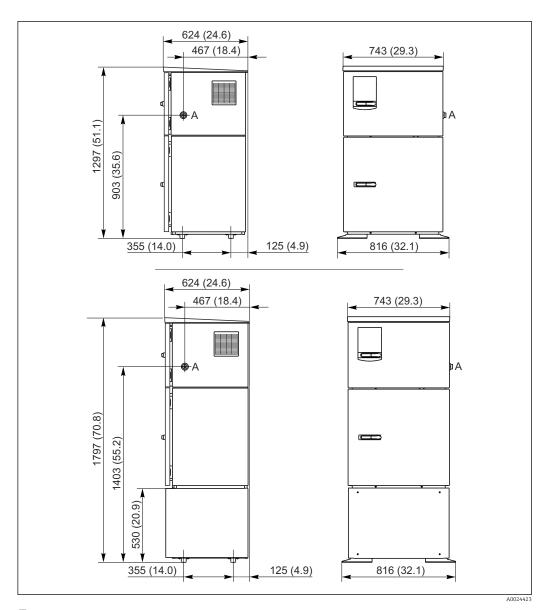
🖻 19 Dimensions of Liquistation, stainless steel version, without/with stand. Unit of measurement mm (in)
