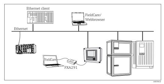
■ 27 Modbus TCP or Ethernet/IP or PROFINET
