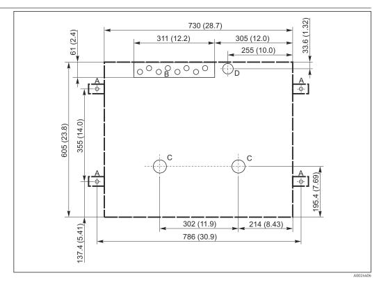
Foundation plan. Unit of measurement mm (in)
