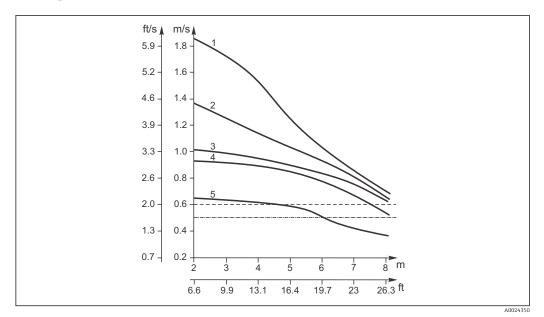
$\blacksquare$  11 Intake speed in m/s (ft/s) with suction height in m (ft)
