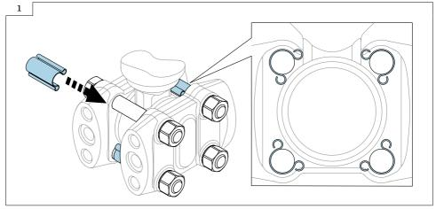
▶ Fit the protective terminal (sacrificial anode) on the screw.
