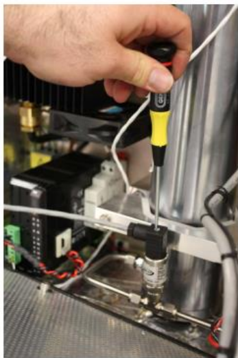
Figure 36. Removing the screw from the harness cap
