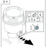
Housing lock for aluminum and stainless steel housing only. Not for plastic and hygienic housing.
