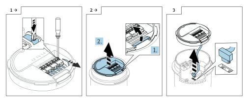
6.2.4 Removing the main electronics
