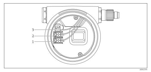
■ 1 Connection terminals and ground terminal in the connection compartment
