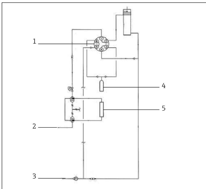
Fig 22. Flow diagram of differential sample system with permeation tube validation
