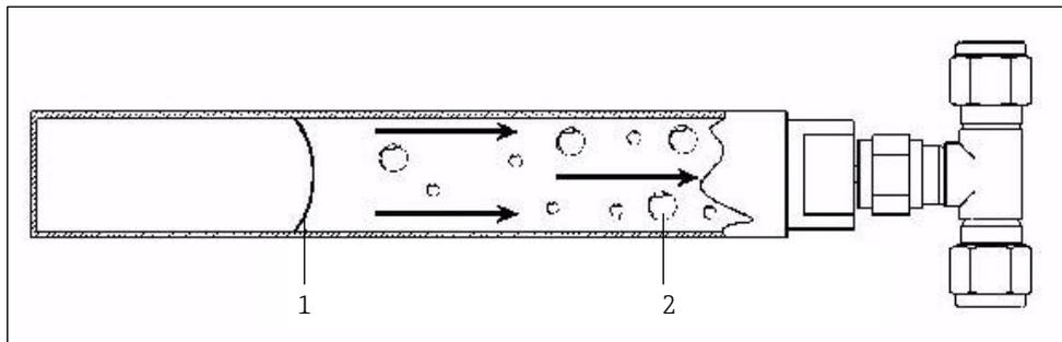
Fig 21. Permeation tube cross section
