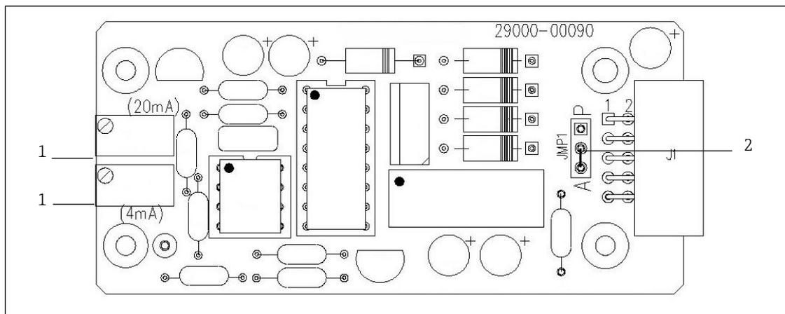
Fig 25. Analyzer 4-20 mA board
