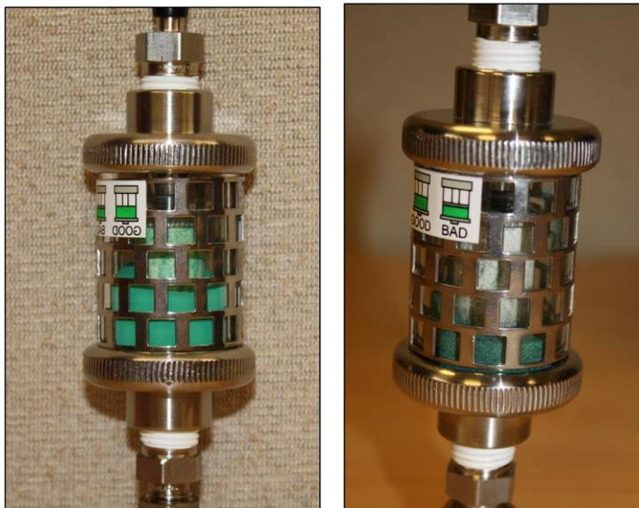
Figs 48 and 49. H<sub>2</sub>S scrubber efficiency indicator before breakthrough (left) and after breakthrough (right)
