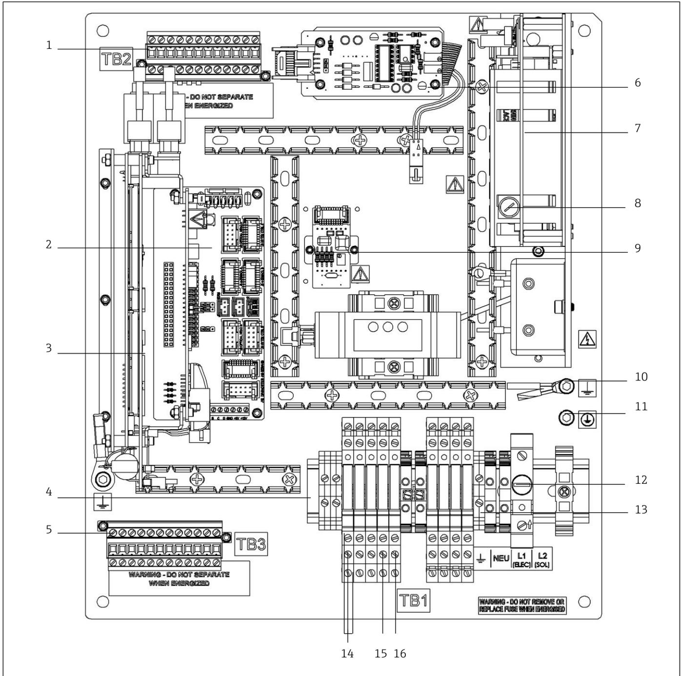
Fig 56. H<sub>2</sub>S analyzer electronics board (DC) showing signal terminal block and alarm relays
