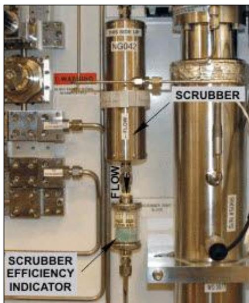
Fig 47. Scrubber and scrubber efficiency indicator
