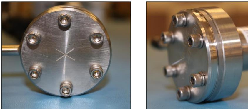
Figs 27 and 28. Stainless steel mirror marking: mirror with engraved X (left), mirror with grooved rim (right)
