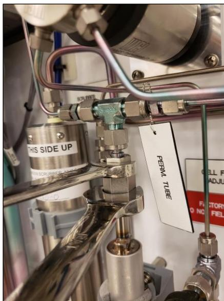
Fig 24. Tightening the perm tube fittings
