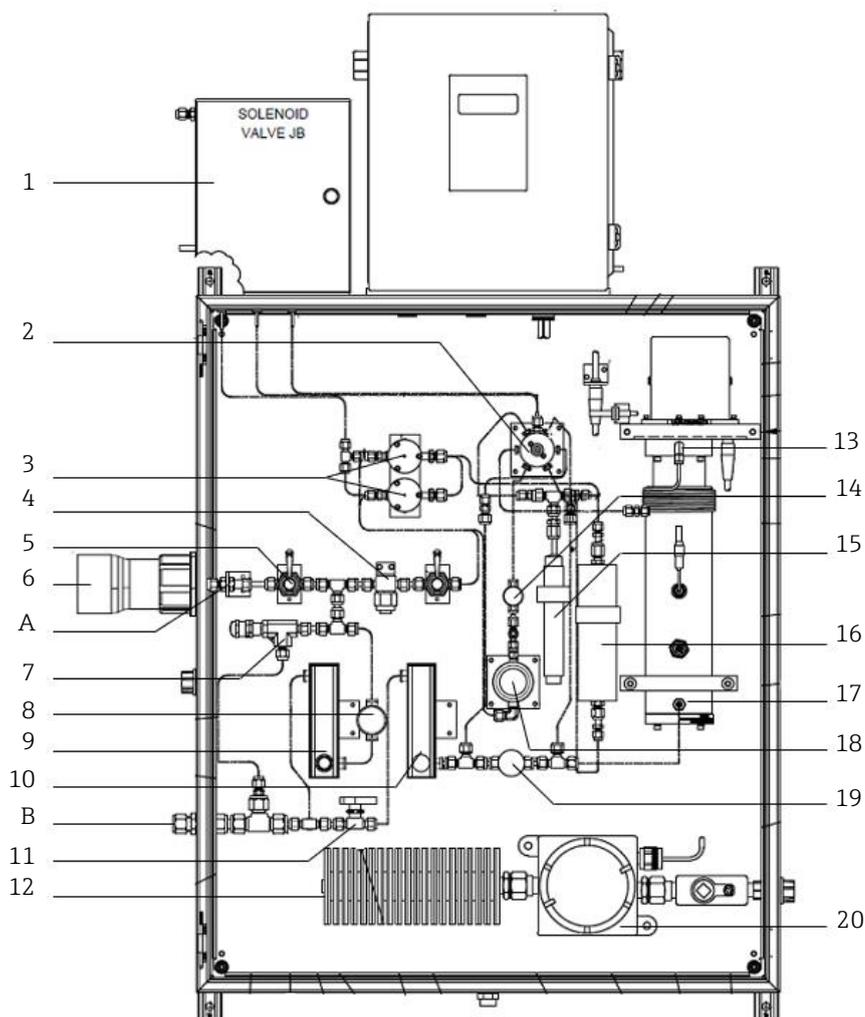
Fig 8. SS2100 analyzer for trace measurements, including H<sub>2</sub>O and NH<sub>3</sub>
