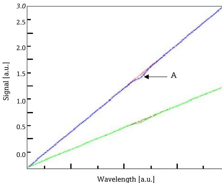
Fig 3. Typical raw signal from a laser diode absorption spectrometer with and without mirror contamination
