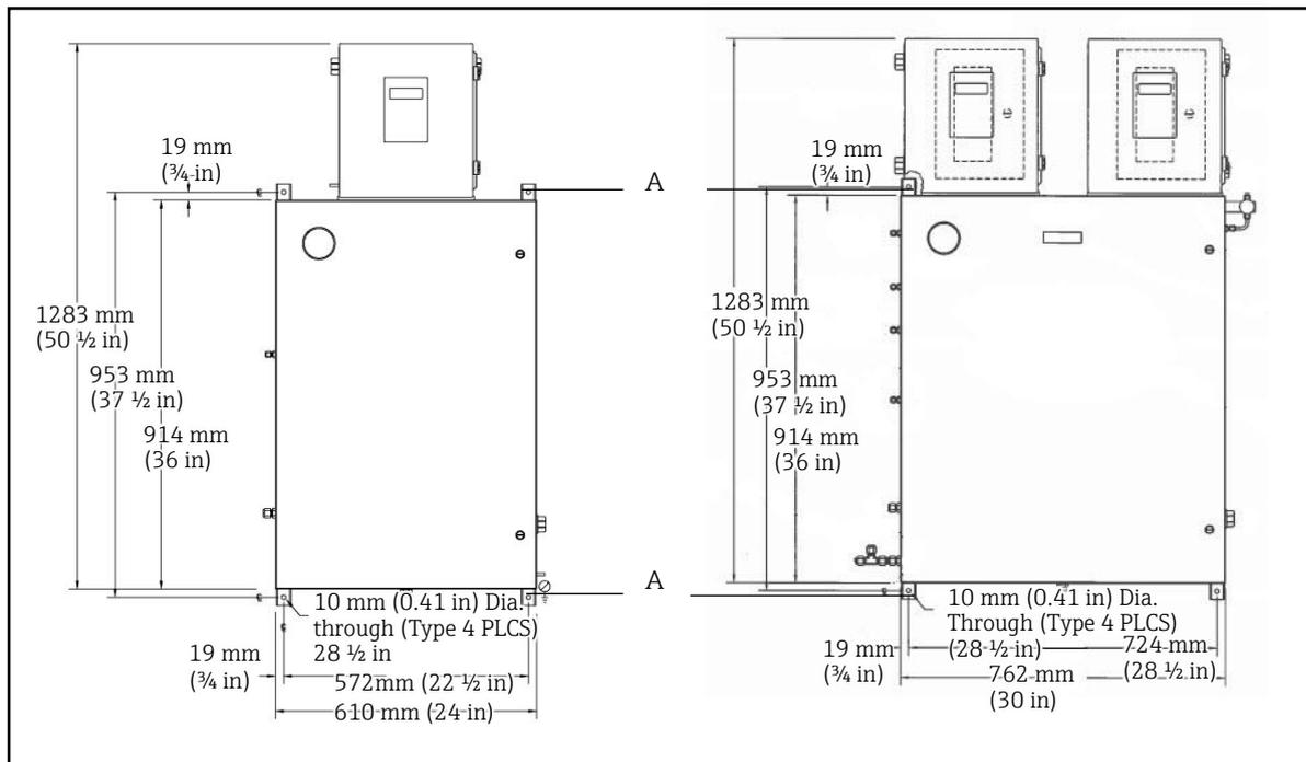
Fig 11. Mounting points for the SS2100 TDLAS Gas Analyzer, designated with A (both sides)
