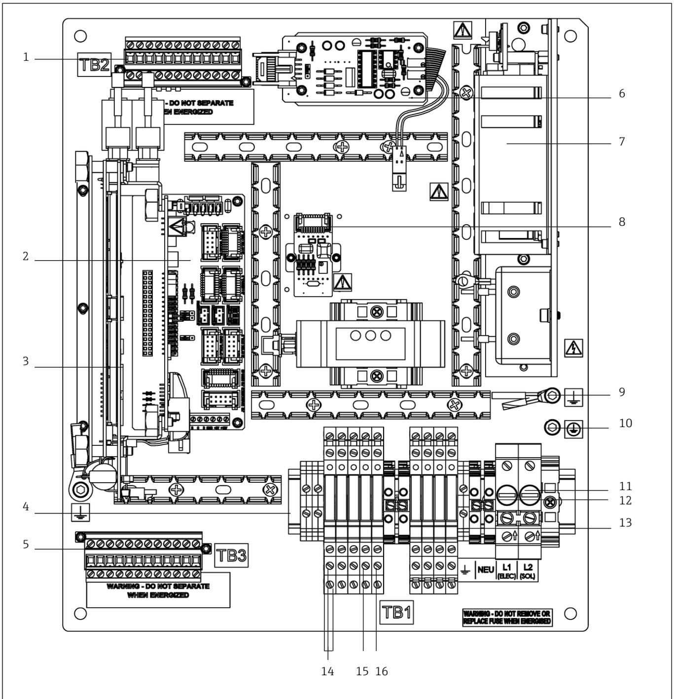
Fig 55. H<sub>2</sub>S analyzer electronics board (AC) showing signal terminal block and alarm relays
