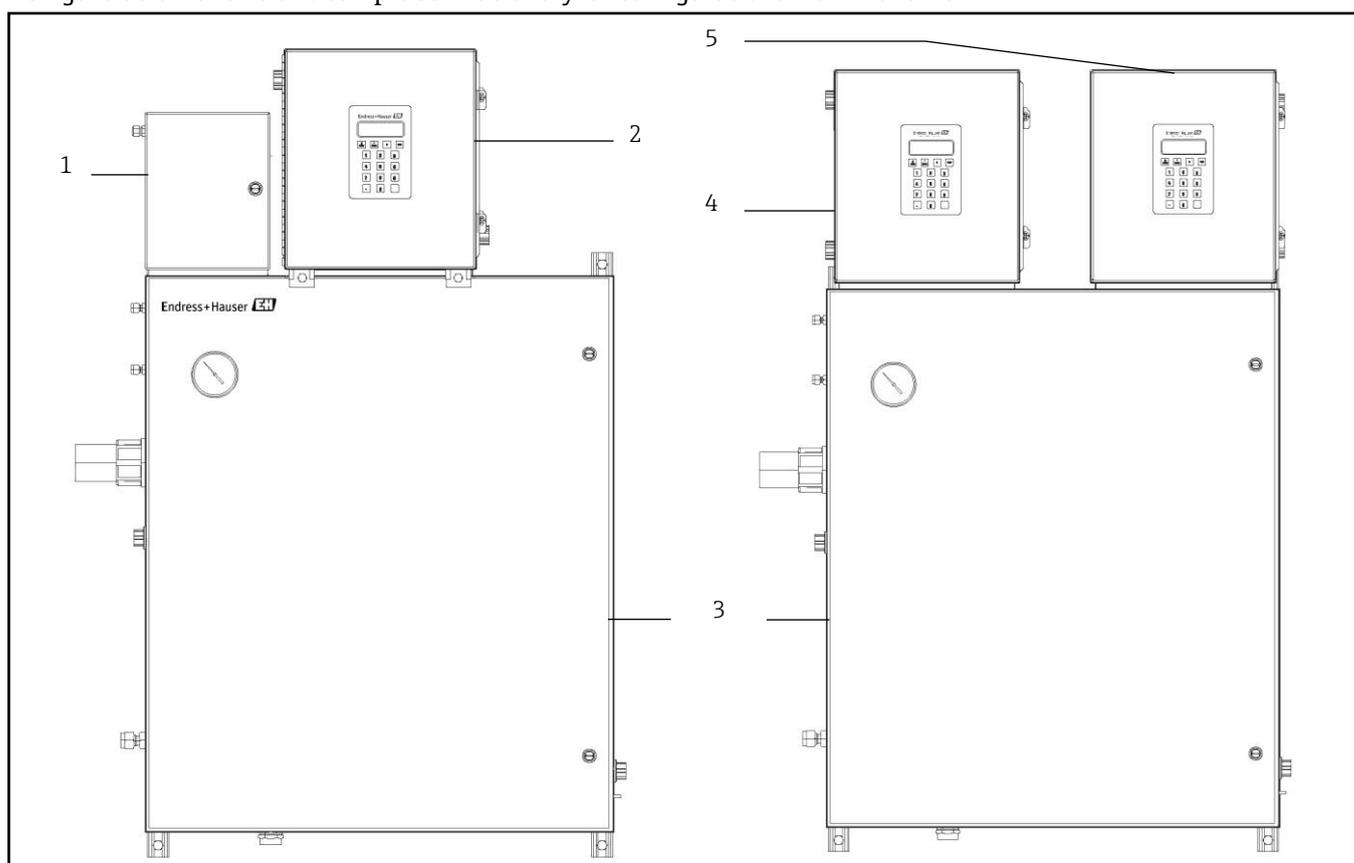
Fig 1. SS2100 TDLAS Gas Analyzer for single analyte (left) and multiple analytes (right), front view
