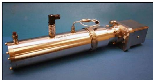
Fig 33. Removed measurement cell with pressure sensor oriented up
