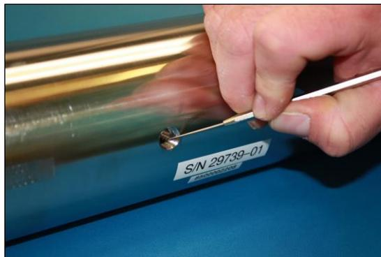
Fig 35. Removing excess seal tape from flange
