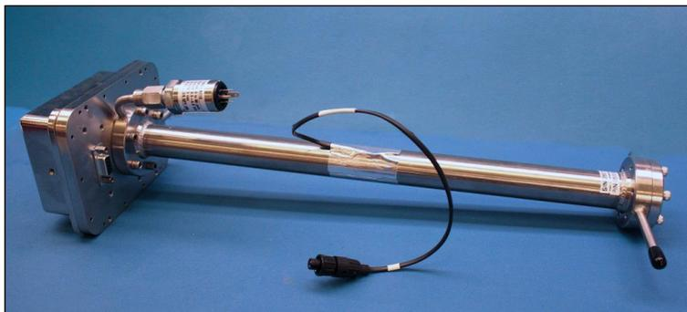
Fig 40. Removed 0.8 m measurement cell with pressure sensor face up
