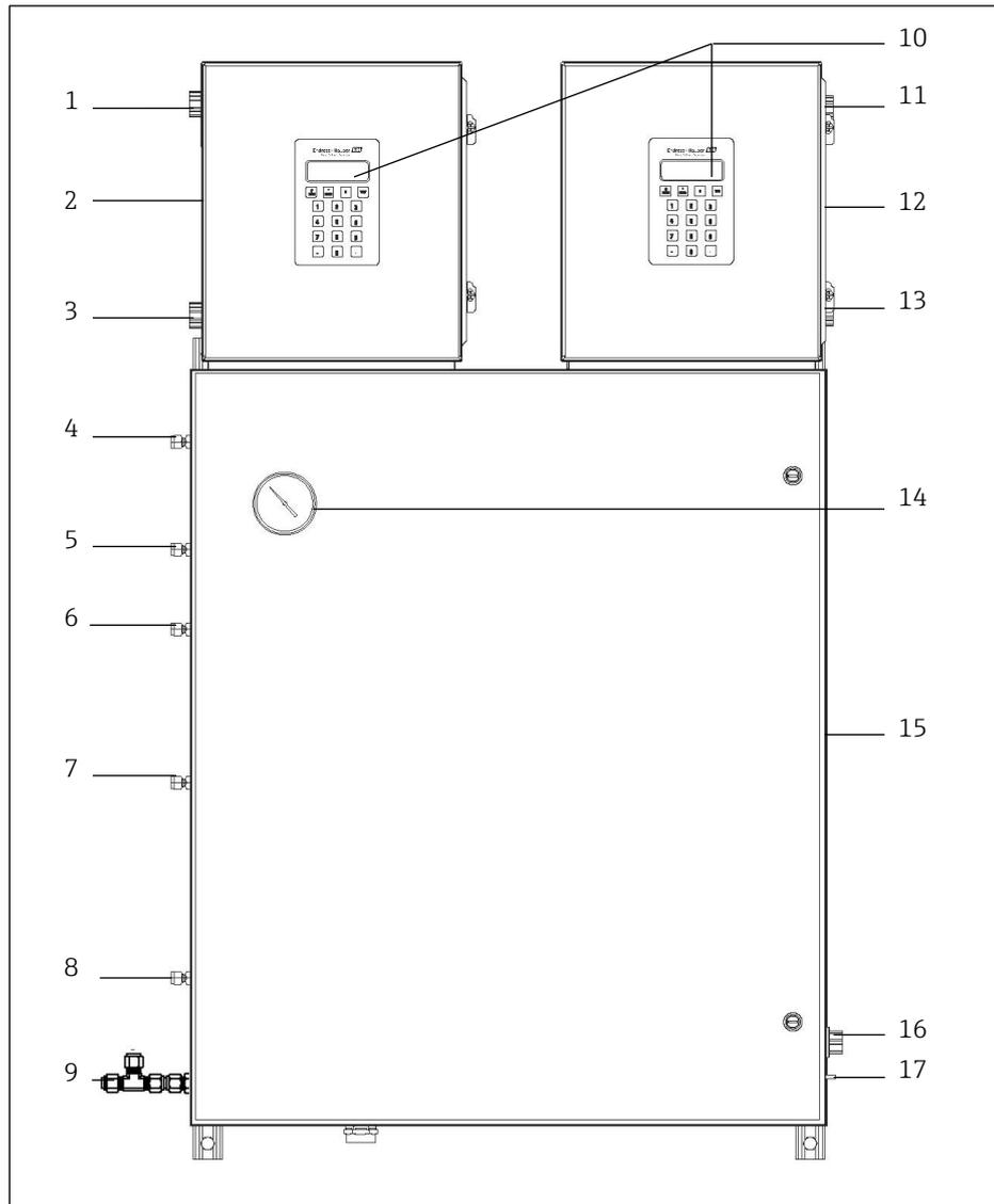
Fig 9. SS2100 2-pack and 3-pack analyzer external structure, front view
