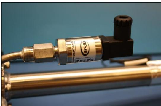
Fig 45. Newly installed pressure sensor positioning
