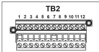
Fig 18. Terminal block TB2 in electronics enclosure for signal cable connection
