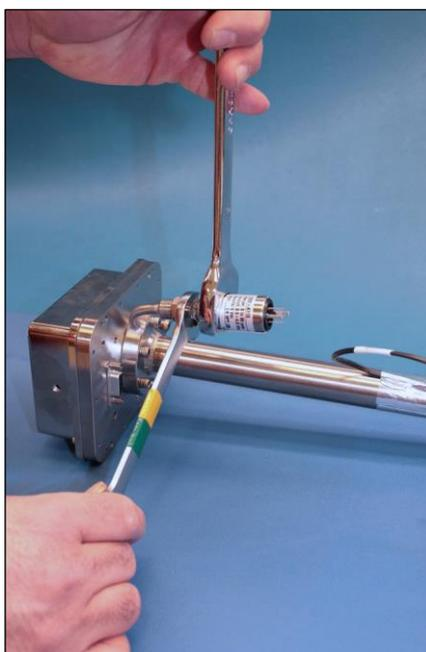
Fig 41. Removing the old pressure sensor
