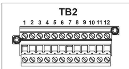
Fig 17. Terminal block TB2 in electronics enclosure for signal cable connection
