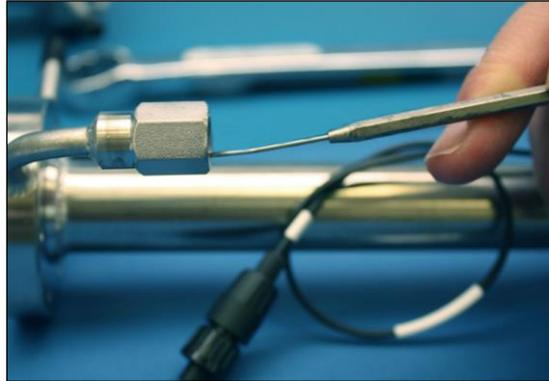
Fig 42. Removing excess seal tape from flange
