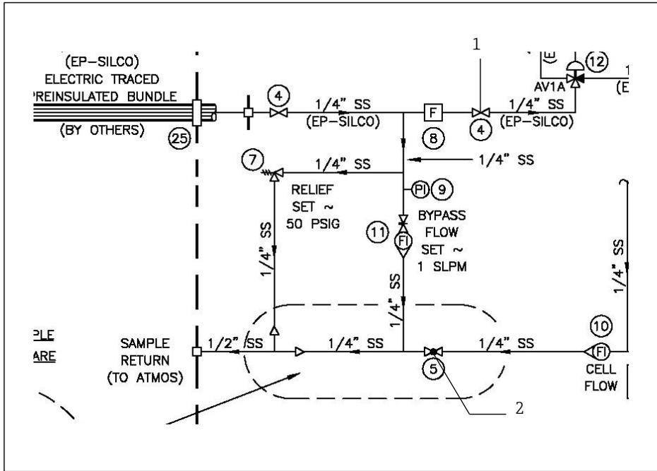
Fig 20. Cell supply and return shut-off valves
