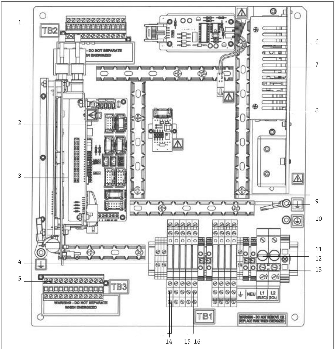
Fig 65. H<sub>2</sub>O, NH<sub>3</sub> analyzer electronics board (AC) showing signal terminal block and alarm relays
