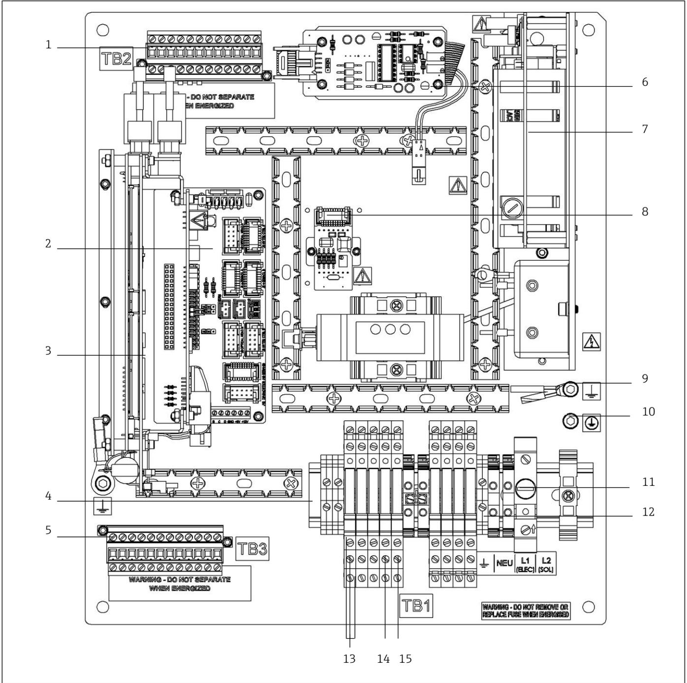
Fig 66. H<sub>2</sub>O, NH<sub>3</sub> analyzer electronics board (DC) showing signal terminal block and alarm relays
