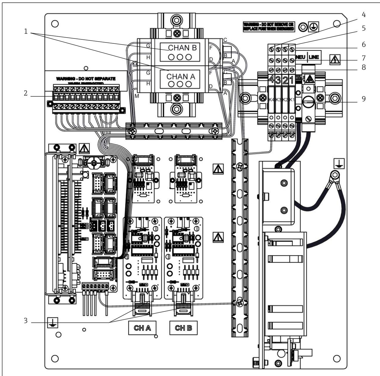
Fig 87. Analyzer B e-series electronics control board (AC) showing signal terminal block and alarm relays with RS-485 communication
