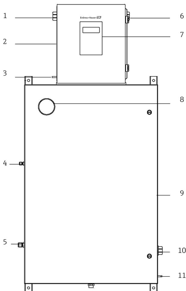
Fig 6. SS2100 non-differential analyzer, front view
