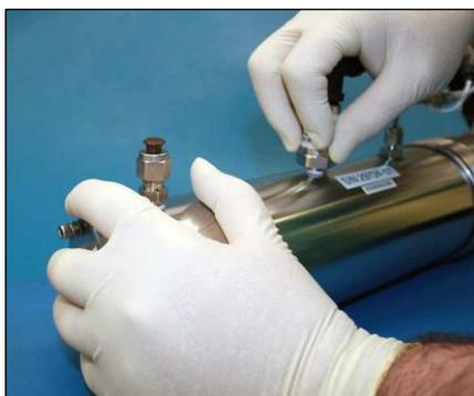
Fig 38. Replacing the pressure sensor
