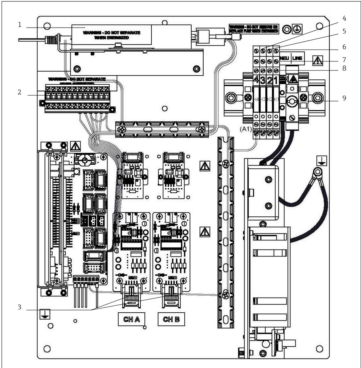
Fig 86. Analyzer B PP2f firmware electronics board (AC) showing signal terminal block and alarm relays with Ethernet connection
