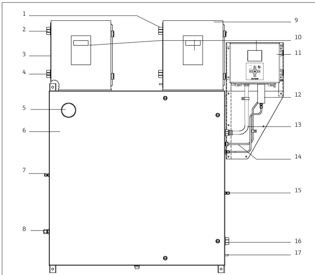
Fig 10. SS2100 2-pack and 3-pack with OXY5500 analyzer external structure, front view
