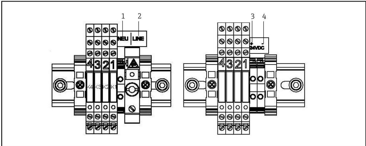
Fig 13. AC (left) and DC (right) connections for the electronics control board terminal block in analyzer B electronics enclosure
