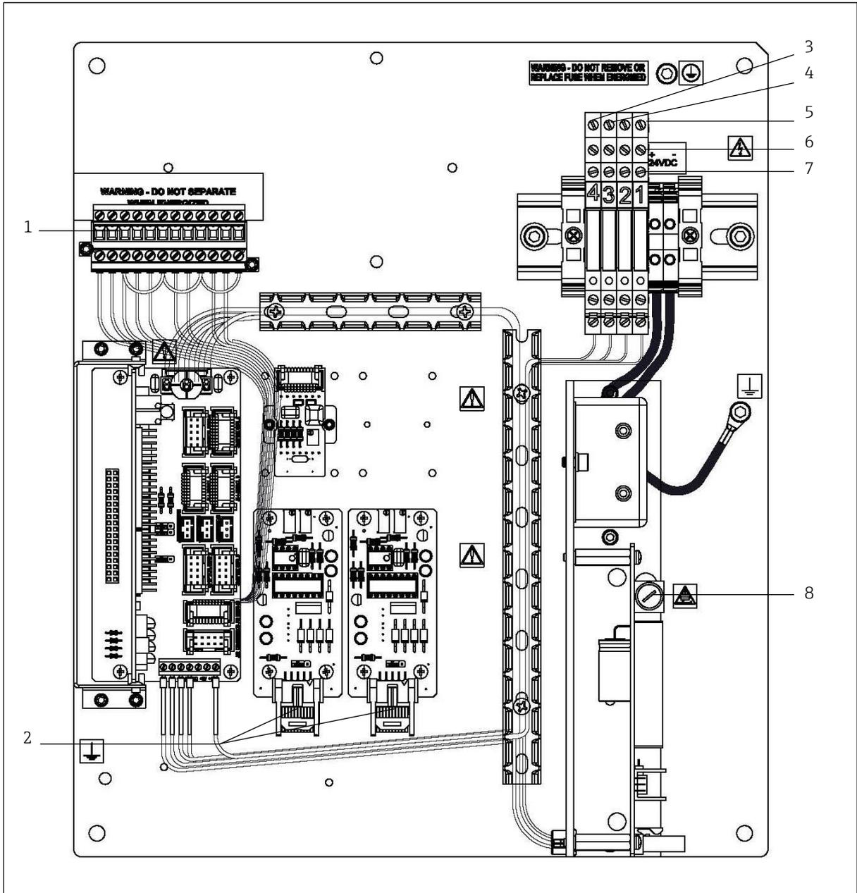
Fig 88. Analyzer B PP2f firmware electronics control board (DC) showing signal terminal block and alarm relays
