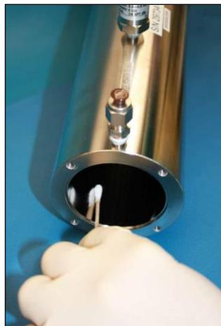
Fig 36. Removing excess seal tape from inside measurement cell
