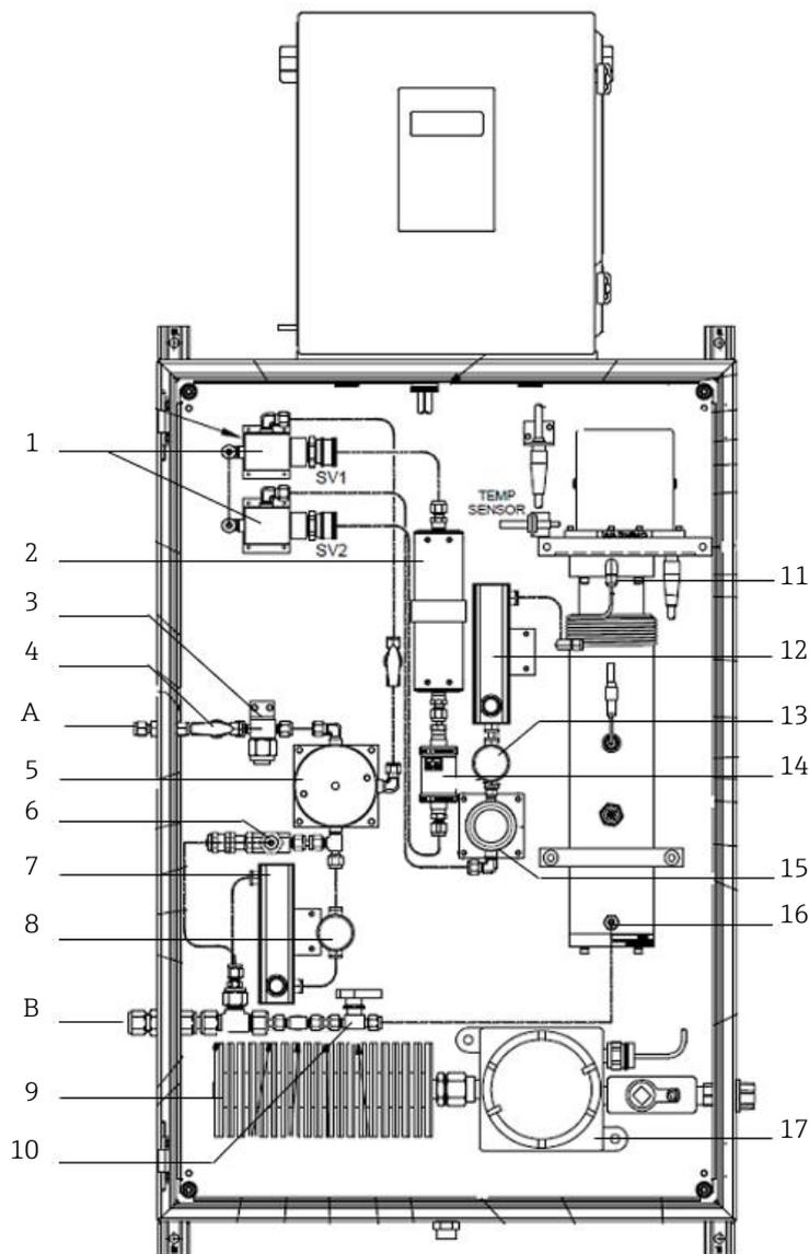
Fig 7. SS2100 analyzer for hydrogen sulfide (H<sub>2</sub>S), front view
