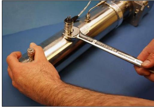
Fig 34. Removing the old pressure sensor
