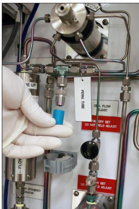
Fig 23. Removing the plug cap for permeation tube installation
