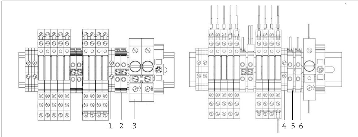
Fig 12. Single phase (120 VAC/240 VAC) connection terminal block (left) and 24 DC connection terminal block (right)
