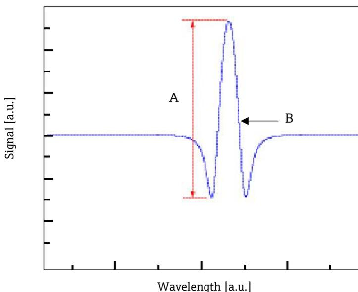
Fig 5. Typical normalized  $2f$  signal showing species concentration proportional to height
