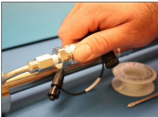
Fig 44. Replacing the pressure sensor
