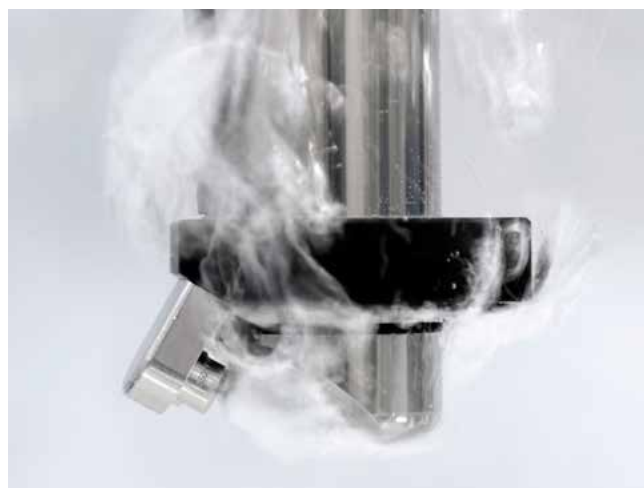
Air cleaning system of the Turbimax CUS52D turbidity sensor
