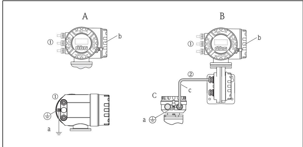
Fig. 3: Design of the measuring system, compact/remote version
