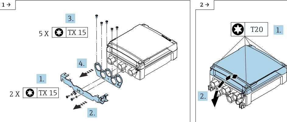
► Loosen the 2 Torx screws and remove the antenna holder. Loosen the 5 Torx screws and remove the conduit adapter.
