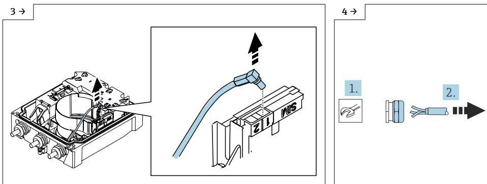
► Disconnect the antenna connector from port 1.
