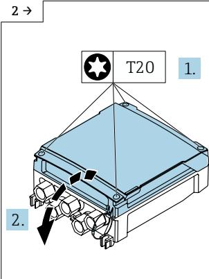
► Loosen the 4 Torx screws on the cover and open the cover.
