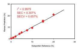
Figure 3: Calibration data for off-line ketoprofen measurements. SEC = Standard error of calibration; SECV = Standard error of cross validation
