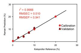
Figure 5: Calibration data for on-line ketoprofen measurements. RMSEC = Root mean squared error of calibration; RMSEP = Root mean squared error of prediction.
