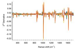
Figure 4: Second derivative spectra for on-line ketoprofen measurements. Several spectra each are included for ketoprofen contents of 2.5%, 5%, 7.5%, 10%, 15%, and 20%.
