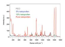
Figure 1: Off-line Raman spectra of ketoprofen films
