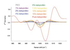
Figure 2: Second-derivative ketoprofen spectra in the spectral area of interest
