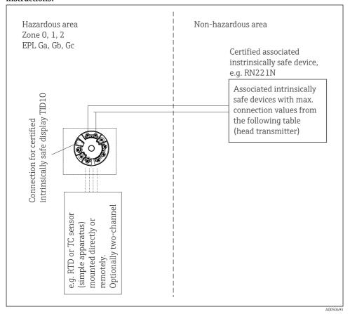
■ 1 Installation of the head transmitter
