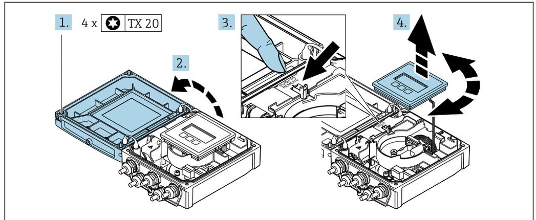
1. Loosen the fixing screws of the housing cover.
