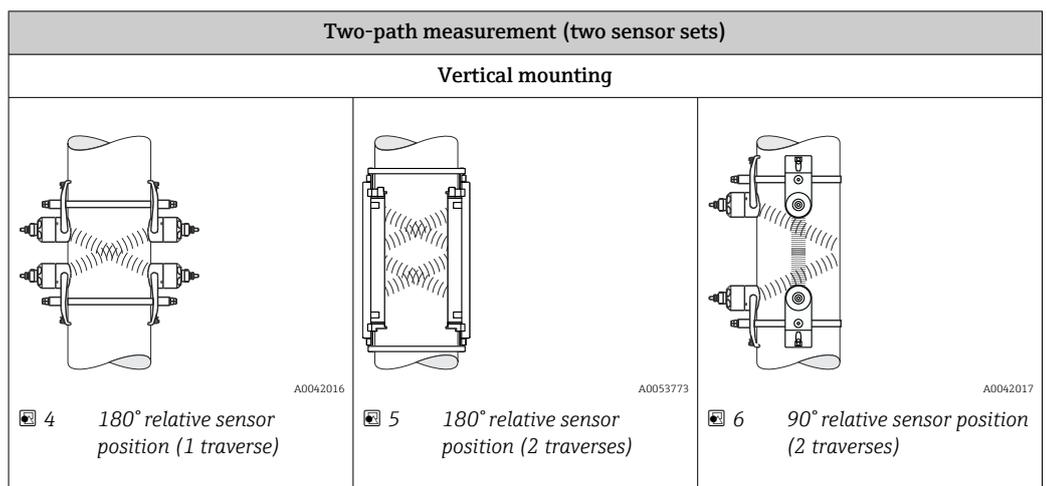
1) Do not swap the sensors of the two sensor sets, as this can affect the measurement performance.
