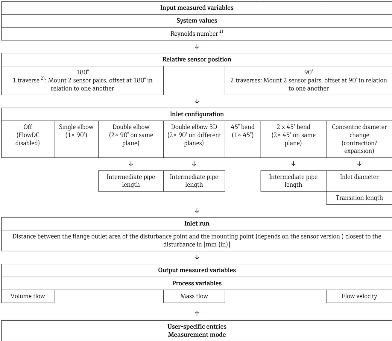
1) Depends on the kinematic viscosity, the average flow velocity calculated and the internal diameter of the measuring pipe
