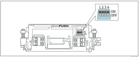
■ 13 DIP switches for hardware-locking of functions
