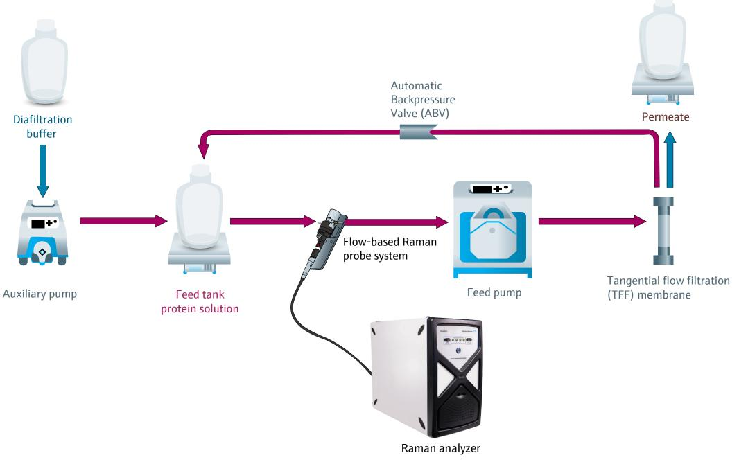
• Diafiltration phase: the volume of the feed tank is maintained at a constant level by continuously adding diafiltration buffer while simultaneously filtering out the process buffer.
