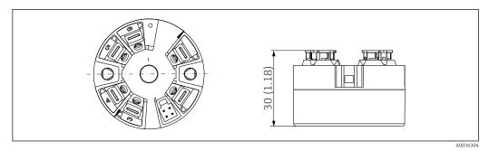
**2**1 € **2**1 Version with push-in terminals. Dimensions are identical to the version with screw terminals, apart from housing height.
