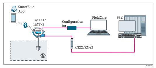
$label{eq:continuous}$  Operation options for the transmitter via the CDI interface
