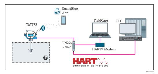
13 Operation options for the transmitter via HART communication
