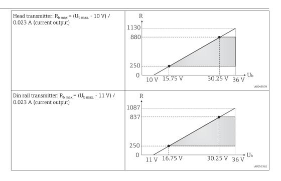
Load in  $\Omega$ .  $U_b$  = supply voltage in V DC
