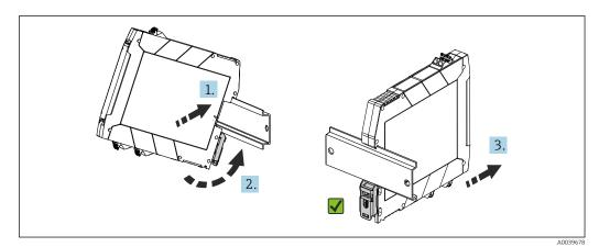
■ 5 Mounting the DIN rail transmitter
