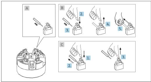
$\blacksquare$  9 Push-in terminal connection, using the example of a head transmitter
