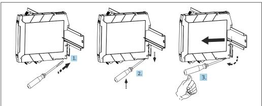
■ 6 Dismantling the DIN rail transmitter
