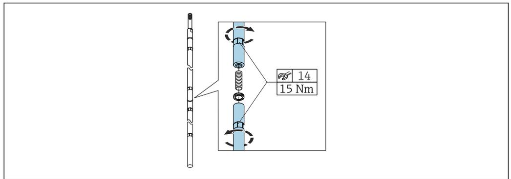
In confined mounting conditions (ceiling clearance), the use of separable rod probe (Ø 16 mm) is advisable.
