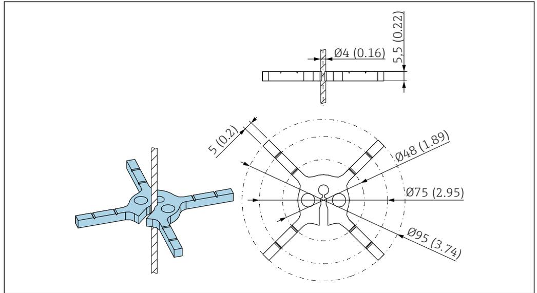
The centering star is suitable for probes with a rope diameter of 4 mm (1/8 in) (including coated rope probes).
