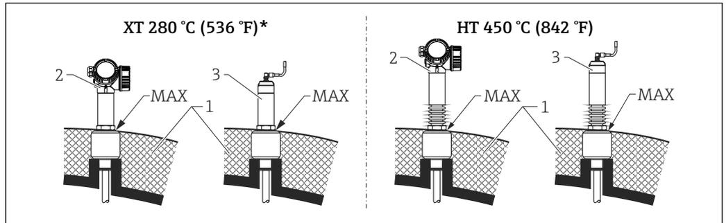
39 Process connection with thread - sensor version XT and HT
