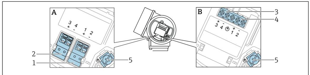
24 Terminal assignment PROFIBUS PA / FOUNDATION Fieldbus
