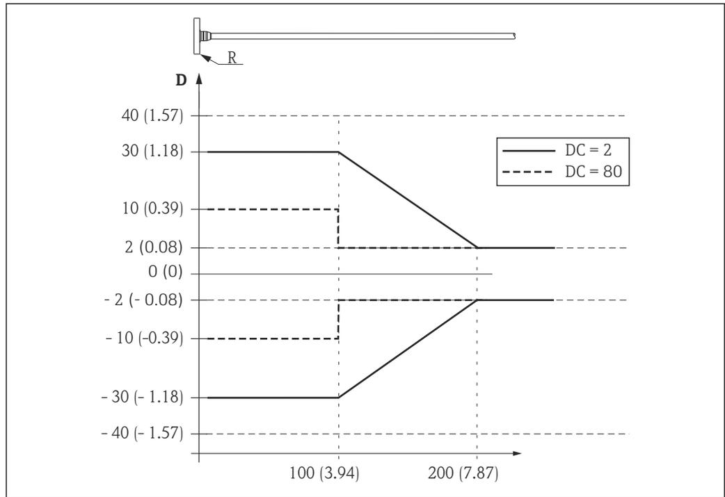
32 Measurement error at the upper probe end; unit: mm (in)
