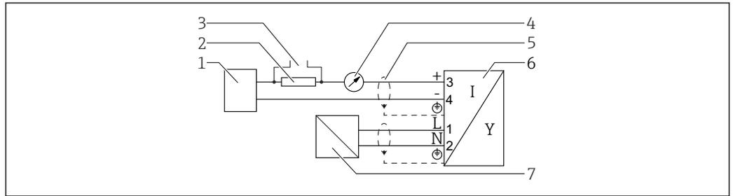
23 Function diagram 4-wire: 4 to 20 mA HART (90 to 253 V<sub>AC</sub>)
