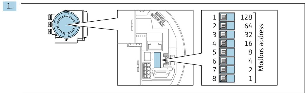
Set the desired device address using the DIP switches in the connection compartment.
